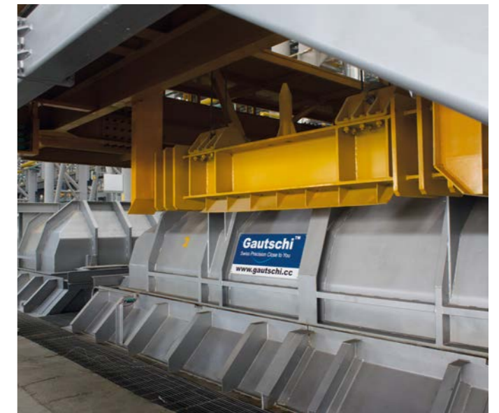
Pit-type furnace to preheat rolling slabs
