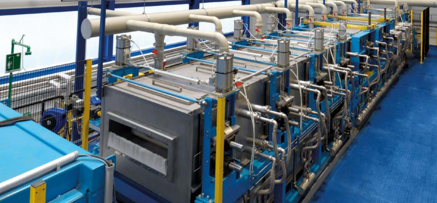
EBNER strip cleaning unit with strip transfer from the rinsing zones to the dryer
