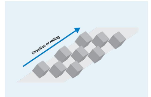
Perfect Goss orientation of the grains in the direction of rolling
