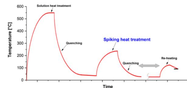
A typical heat treatment profile for AA6xxx strip during processing in a CASH line with additional spiking heat treatment
