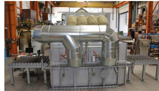
A prototype roller-hearth furnace for aluminum hot forming
