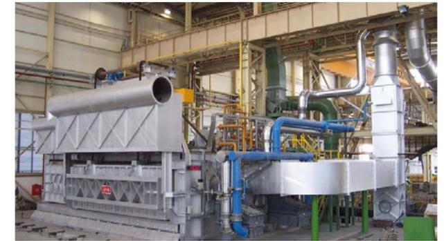
The completed shell of the 145 t dual-chamber melting furnace
