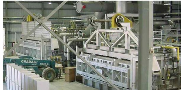
A pivoting 50 t scrap melting and holding furnace
