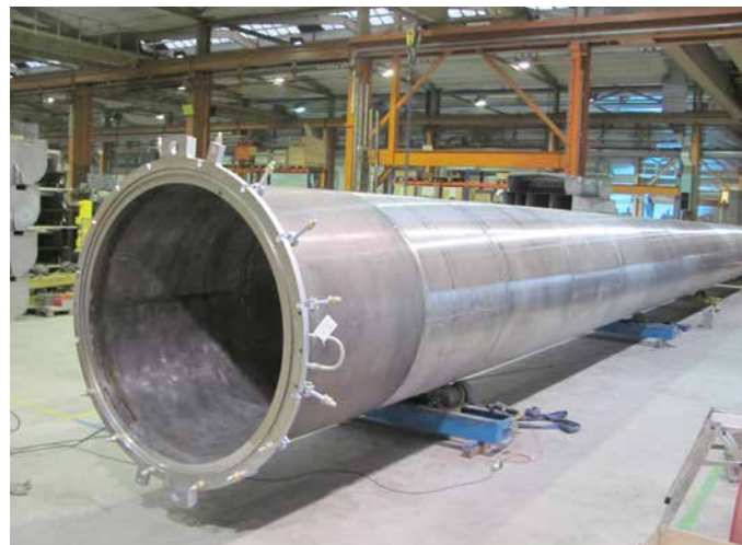
Muffle in the EBNER workshop
