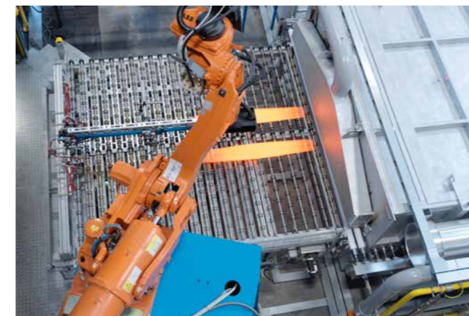
Red-hot blanks ready for the press
